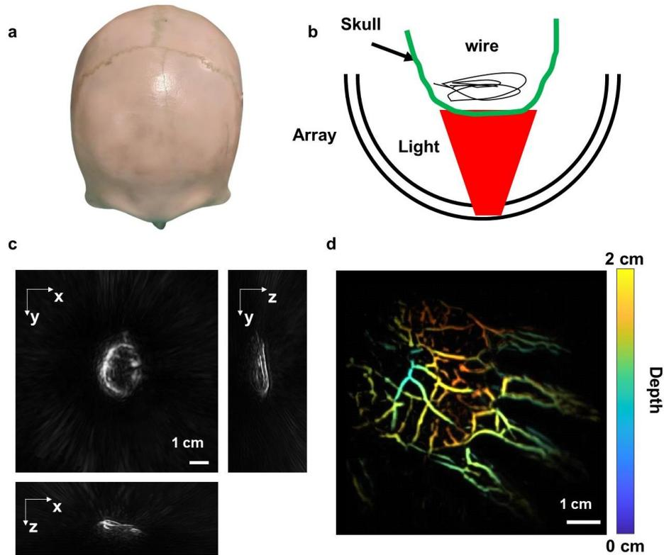
**Figure 5. Demonstration of transcranial 3D PACT imaging and fast *in vivo* imaging.** **a** Photo of human skull from a donor used in the phantom study. **b** Schematic of the *ex vivo* transcranial imaging experiment. **c** Transcranial images of the wire. **d** Depth-encoded *in vivo* image of a human hand.
