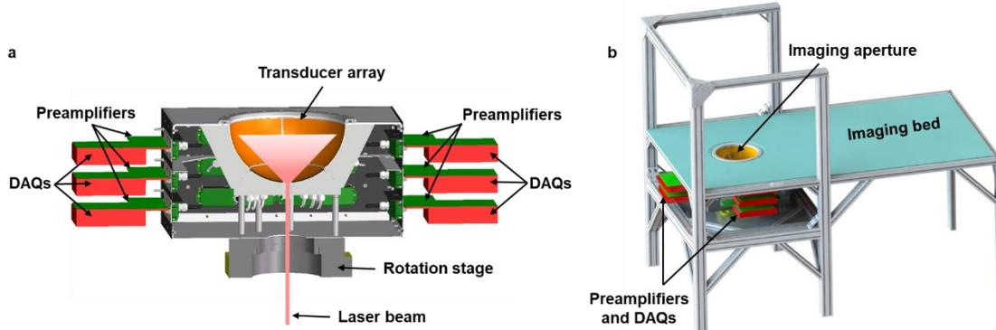
**Figure 1. Representations of the 3K-PACT. a** Cut-away view of the 3K-PACT imager. **b** Perspective view of the 3K-PACT system. DAQ, data acquisition module.
