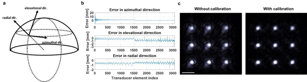
**Figure 2. Geometric calibration of the 3K-PACT array.** **a** Representation of three directions in the array geometric calibration. **b** Errors segmentation into azimuthal, elevational, and radial directions. **c** Reconstruction of a scanned point source pattern using designed element positions and calibrated element positions. Scale bar, 5 mm.
