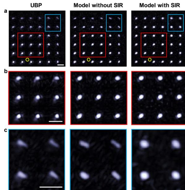
**Figure 3. Comparison between different reconstruction methods.** **a**  $XY$  projection images of 3D PACT reconstruction of a  $6 \times 6$  point source pattern by UBP, model-based iterative reconstruction without SIR and with SIR. The yellow circles indicate the transducer array center position. **b** Close-up images near the center to show reconstruction artifacts. **c** Close-up images near the edge to show reconstruction distortions. Scale bars, 5 mm.
