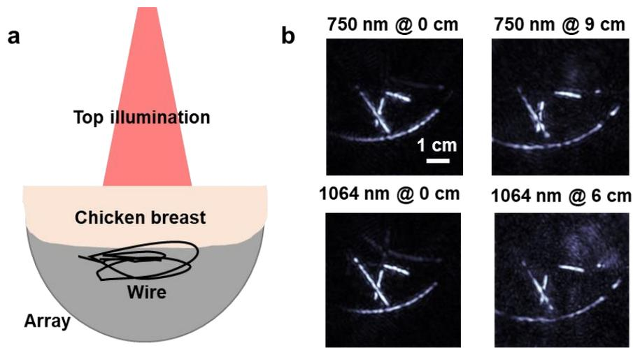
**Figure 4. Single-shot PACT imaging through *ex vivo* tissue of varying thicknesses.** **a** Schematic of the experiments. **b** Single-shot PACT images acquired without and with chicken breast tissues of different thicknesses with 750 nm and 1064 nm lasers, respectively.
